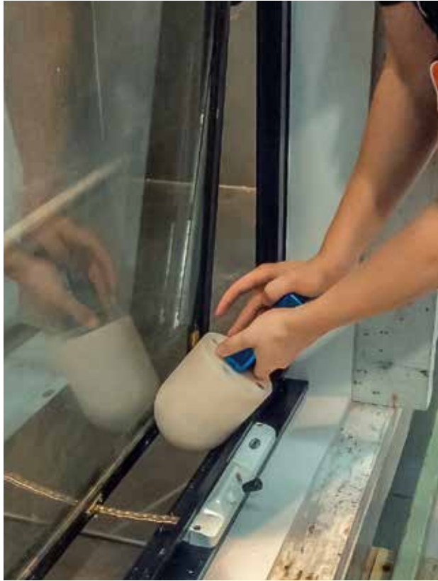
Fall Prevention testing on Dowell Awning and Sliding windows
