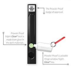
The key has been designed with Night-Glow® materials, to assist you should you need to find the key in the dark. The luminescent material is a 1:1 charging: emitting ratio, up to 8 hours, so if the key is in the sun during the day and absorbs light for 8 hours, it will glow, declining in brightness over the time, for 8 hours.
