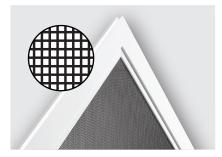
Force Field® features black powder coated, 316 marine grade stainless steel mesh. The 0.8mm diameter wire has a 1.62mm aperture providing an open area of 42.5%, for excellent visibility, airflow and compliance to
